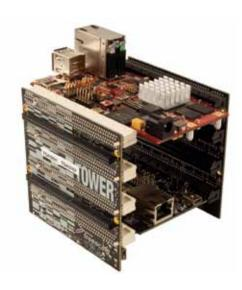
The partnership of Freescale, QNX®, ISaGRAF® and koenig-pa GmbH (KPA) provides a programmable logic controller reference platform for easier industrial control system development.
